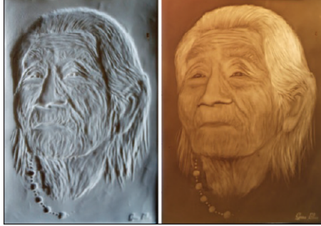
The magic of the lithophane is its ability to change its appearance when illuminated from behind. On the left of this modern lithophane is the image as it appears in reflected light. On the right is how it comes into view as a three-dimensional portrait when made translucent. Photo illustration: Jay Mark
